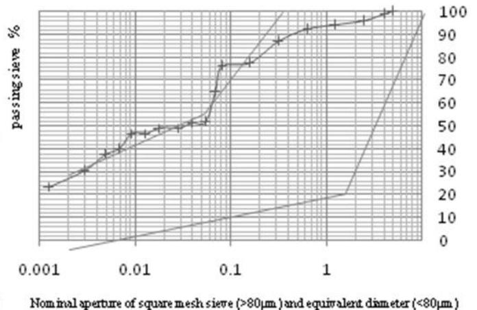
Fig1: Grading curve of the soil (by screening and sedimentation methods).
