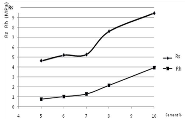
**Fig 2: Influence of cement content on the dry and wet compressive strength Rs, Rh**
