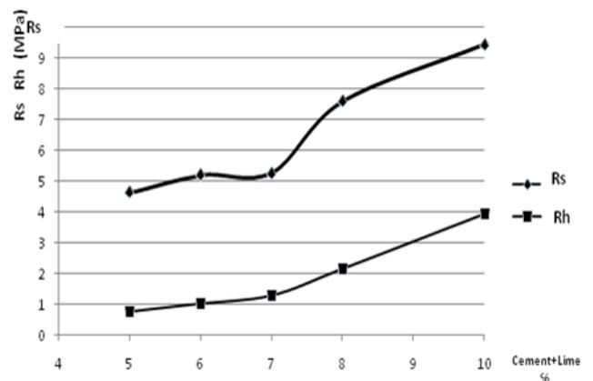
**Fig 4: Influence of cement+lime content on the dry and wet compressive strength Rs, Rh**
