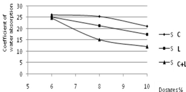
Fig 7: Coefficient of water absorption by capillary versus dosages in Cement(C), Lime (L) and mix of Cement+Lime (CL).
