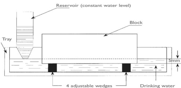
Fig 6: Measure of absorption by capillary [6].
