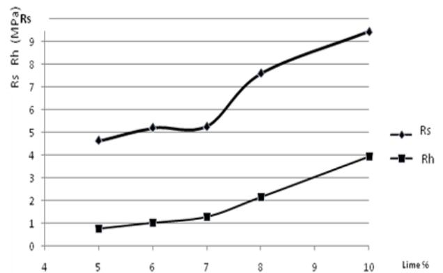
**Fig 3: Influence of lime content on the dry and wet compressive strength Rs, Rh**
