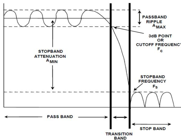
**Fig: 7 Specification of the transmission characteristics of a low pass filter [7].**
