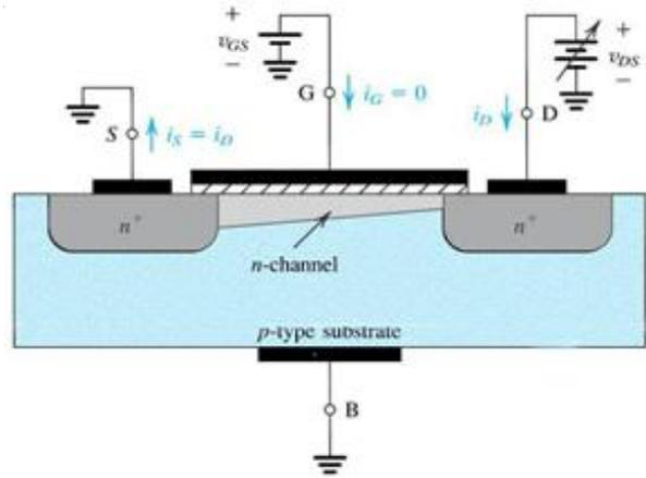
Fig 3: Operation of the enhancement NMOS transistor as  $v_{DS}$  is increased [3].
