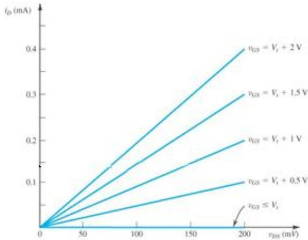
Fig 2:  $i_D$ - $v_{DS}$  characteristics of the MOSFET [2]
