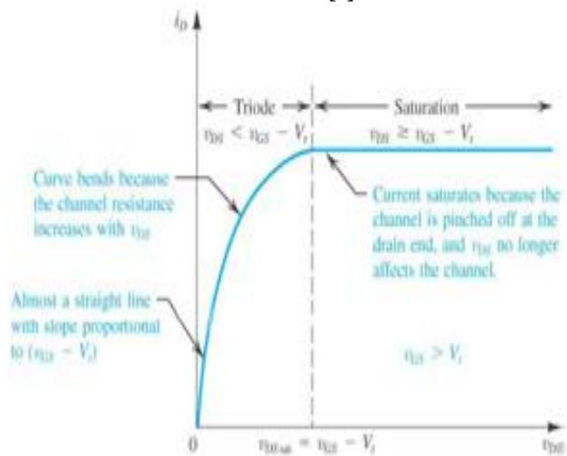
Fig 4:  $i_D$  versus  $v_{DS}$  for an enhancement-type NMOS [4].
