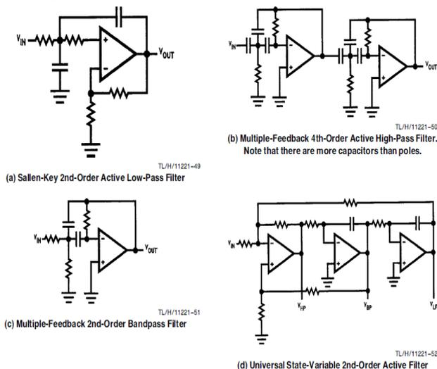
Fig: 8 Examples of Active Filter Circuits Based on Op Amps, Resistors, and Capacitor.
