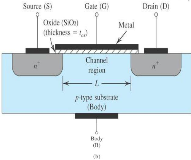
Fig 1: Physical structure of the enhancement-type NMOS transistor: (a) perspective view; (b) cross-section [1].
