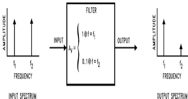
**Fig: 6 Using a Filter to Reduce the Effect of an Undesired Signal [6]**
