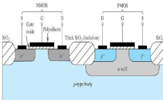
Fig 5 Cross-section of a CMOS integrated circuit [5]
