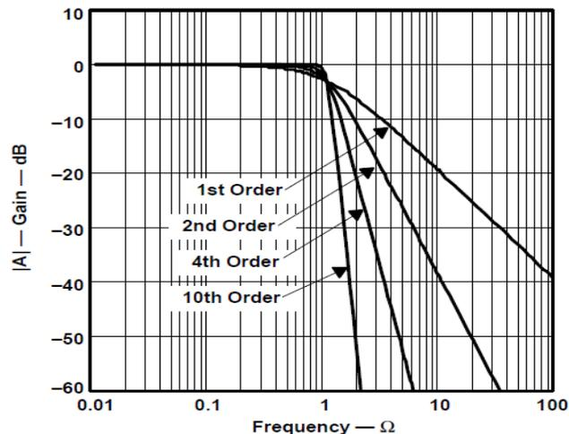
Fig: 9 Amplitude Responses of Butterworth Low-Pass Filters
