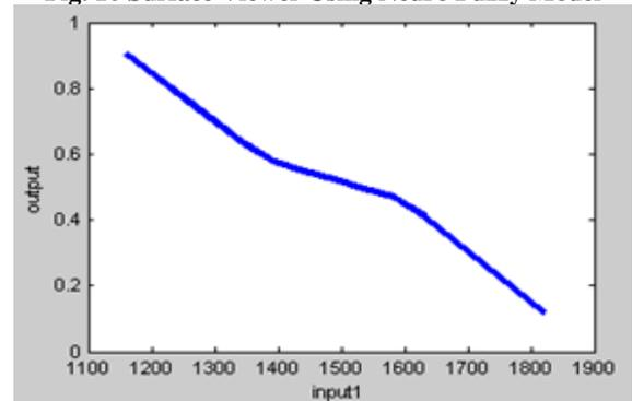
Fig. 11 Relationship between Output (Voltage) With Input1 (Load) For Neuro Fuzzy Model.
