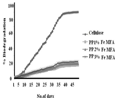
**Fig.12: Bio-degradation curve of PP films in presence of 1%, 3%, and 5% Fe MFA**
