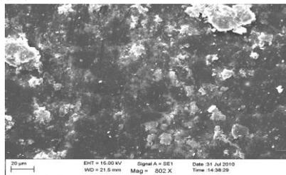
**Fig .11: Effect of MFA on Morphology 3% PP-Fe MFA in the presence of One day (D1) on UV exposure.**
