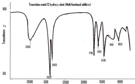
**Fig. 4: FTIR spectra of MFA (Ferrous 12 Hydroxyl oleate)**
