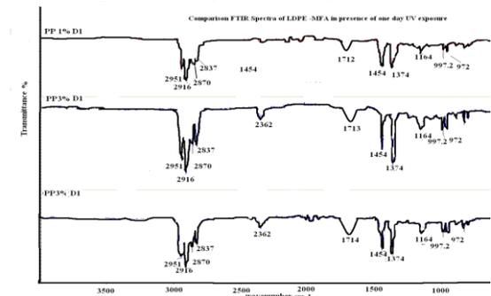
**Fig.6: Comparison FTIR spectra of PP- Fe MFA in presence of one day UV Exposure**
