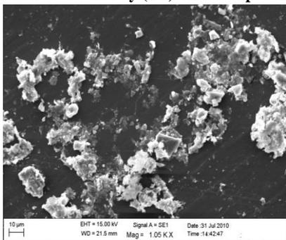
**Fig.10: Effect of MFA on morphology 2%PP-Fe MFA in the presence of one day (D1) on UV exposure**
