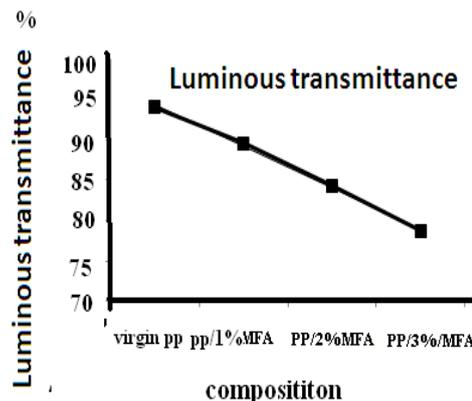
**Fig. 3: Effect of MFA on Luminous Transmittance PP- Fe MFA in Presence of UV Exposure in Presence of UV Exposure.**
