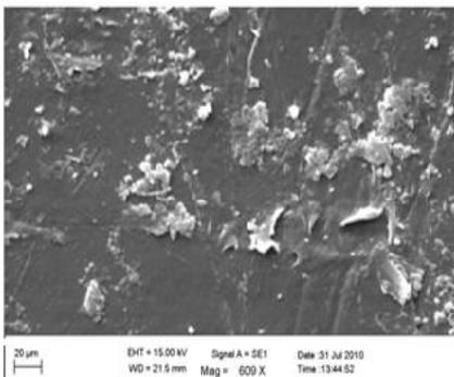
**Fig.8: Effect of MFA on Morphology 3% PP- Fe MFA without UV exposure**
