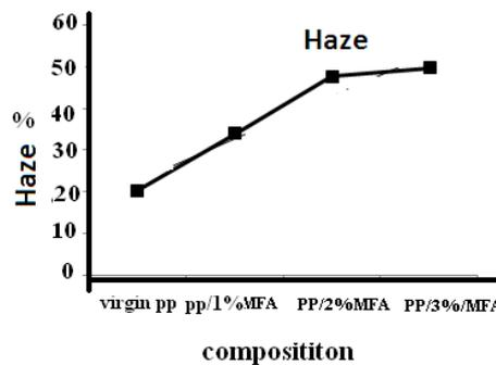
**Fig. 2: Effect of MFA on Haze PP- Fe MFA in presence of UV exposure**
