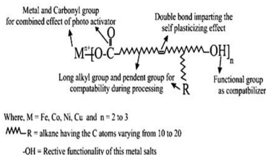
Fig. 1: Generic Structure of Multi Functional Additive (MFA).
