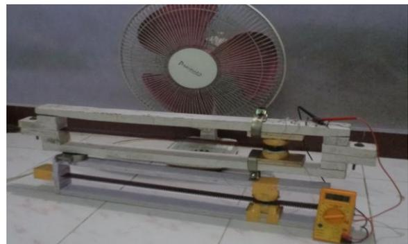
Fig 7 Two Wind Belt Connected In Series
