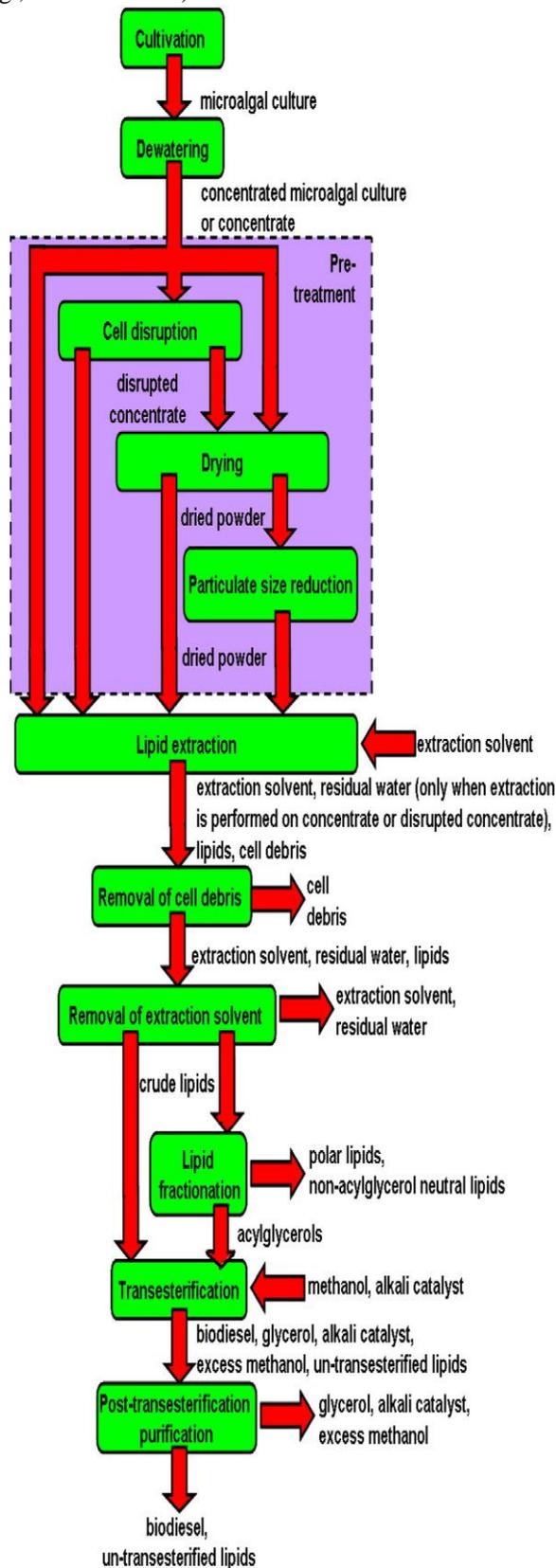
Fig 1 Process flow diagram showing the downstream processing steps needed to produce biodiesel from microalgal biomass.
