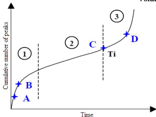
Fig 6. Cumulative Number of Peaks with Creep Test
