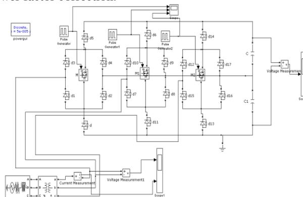
Fig.2 simulation model of Vienna rectifier
