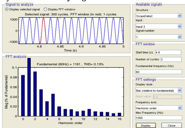
Fig.4 THD Analysis of three phase Vienna rectifiers
