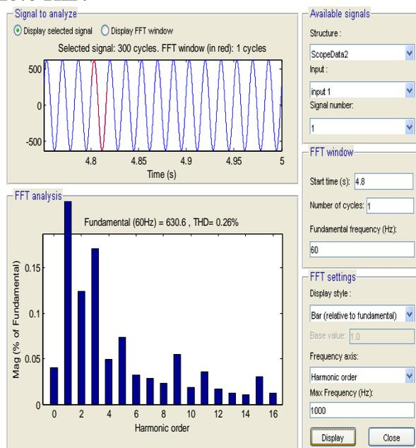
Fig.3 THD Analysis of three phase Vienna rectifier
