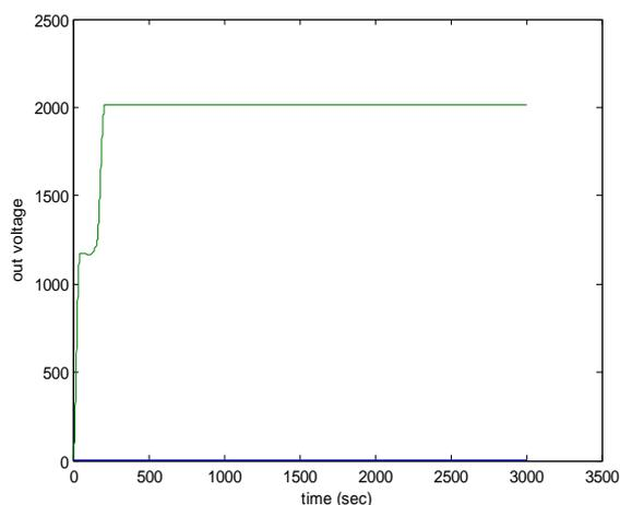
Fig 5 output voltage waveform of three phase Vienna rectifier
