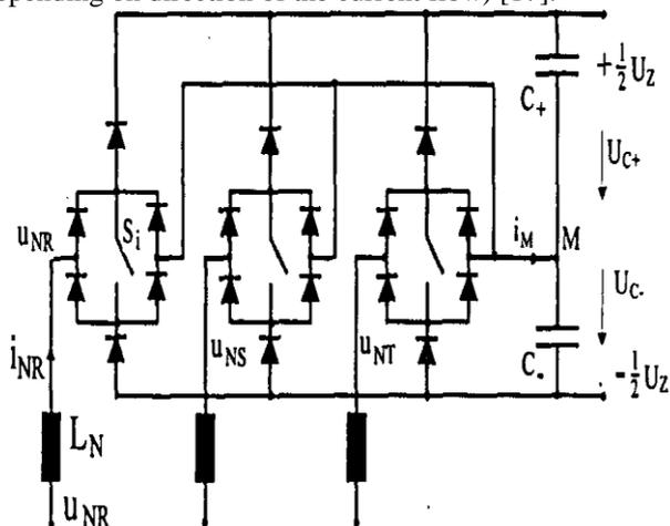
Fig.1 Structure of the power circuit of Vienna rectifier
