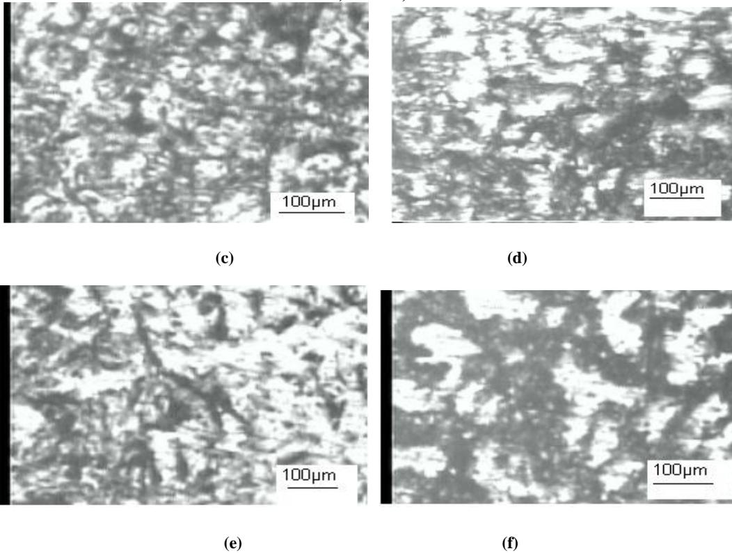
**Fig 3(A) & (B): Microstructure of Al-6.5wt%Si-20wt%Pb Alloy at One Ant Two Third Heights Respectively. (C) & (D): Microstructure of Al-6.5wt%Si-25wt%Pb Alloy at One Ant Two Third Heights Respectively. (E) & (F): Microstructure of Al-6.5wt%Si-30wt%Pb Alloy at One Ant Two Third Heights Respectively.**
