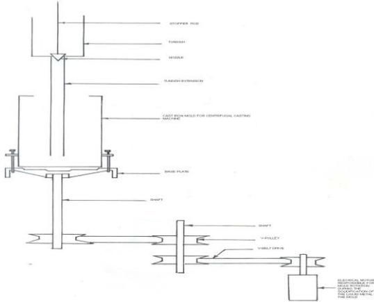
**Fig 2: Vertical Centrifugal Casting Machine**
