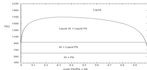
Fig 1: Aluminum- Lead phase diagram
