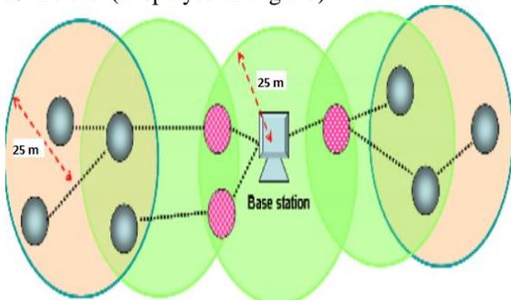
(A) Scenario1: The Base Station and All Sensor Nodes Have The Same Transmission Range.
