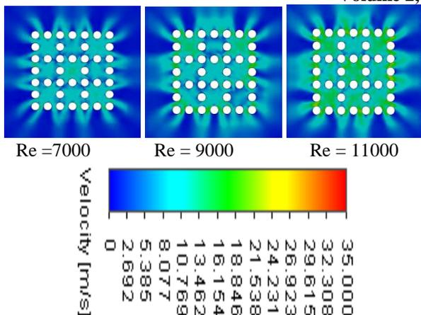
Fig 4 Velocity contours along the horizontal plane 1mm above base plate (Re = 7000-11000).
