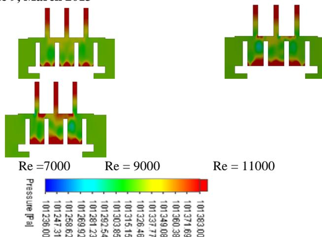
Fig 6 Pressure Contours for Re = 7000-11000
