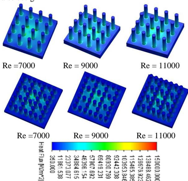
Fig 8 shows the variation of heat flux for sparse and dense designs at  $Re = 7000$  to  $11000$ .
