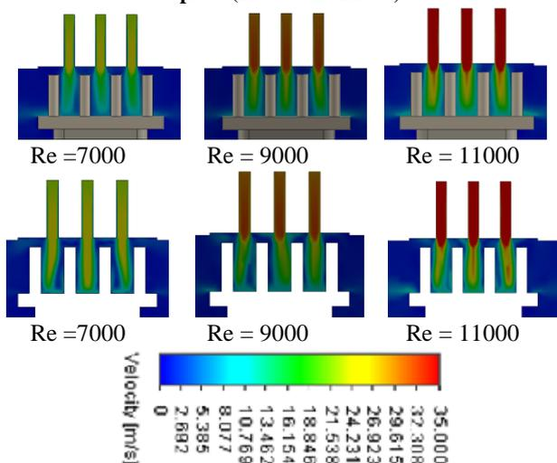
Fig 5 Velocity contours along the Diagonal Vertical plane (Re = 7000-11000)
