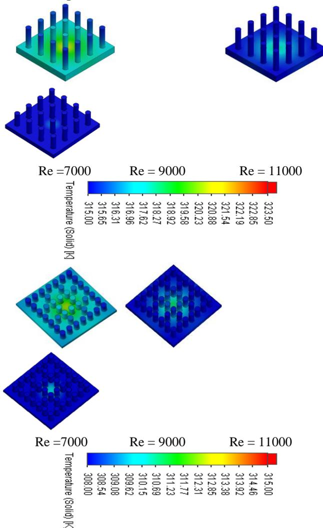
Fig 7 Temperature Contours (Re = 7000-11000)
