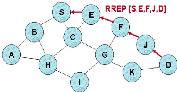
Fig 6. RREP Is Sent By Node D and Path is Setup
