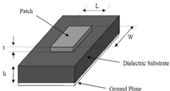
Fig 1: Microstrip patch antenna [6]
