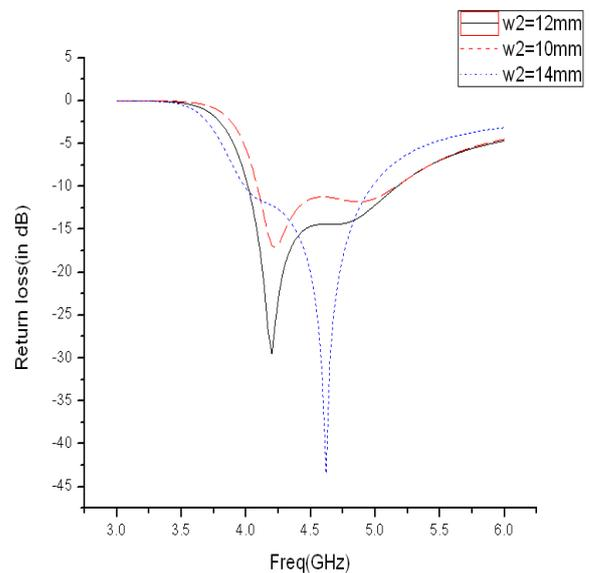
**Fig 7: S-Parameter compared by varying slot width w2 [7]**
