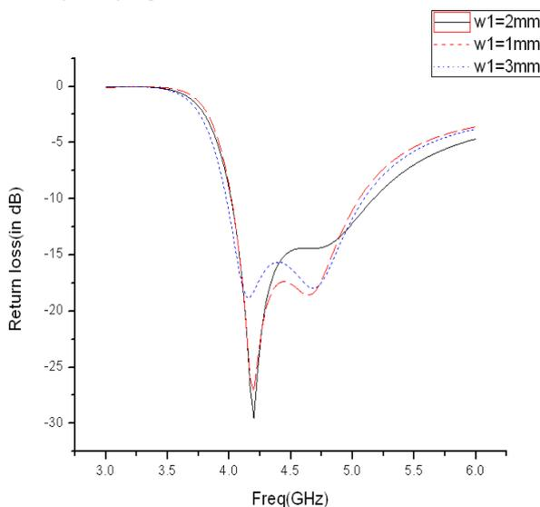
**Fig 5: S-Parameter compared by varying slot width w1 [7]**
