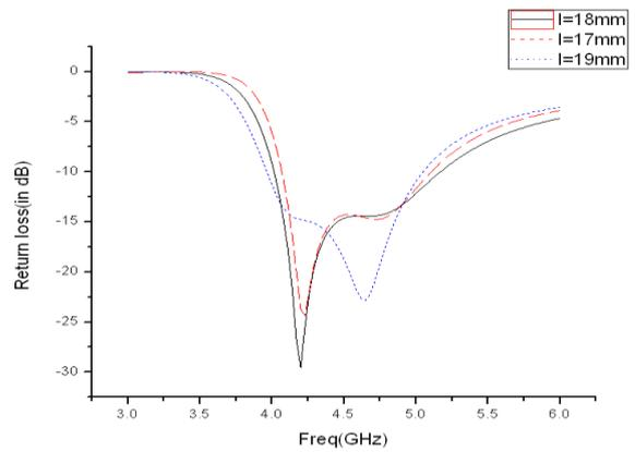
**Fig 6: S-Parameter compared by varying slot length l [7]**
