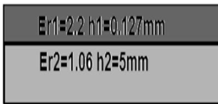
**Fig 4: Substrate Dimensions [7]**
