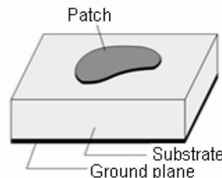
Fig 2: Patch antenna [4]
