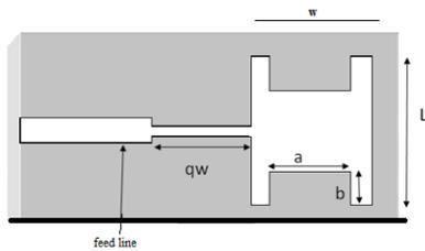
Fig 3: Patch antenna [3]
