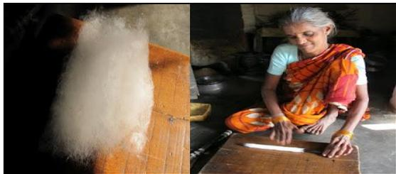
Fig. 1 - manual method of producing Sliver (Pelu).
