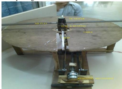
This assembly is attach to the main carding dram with help of duct & due to the high velocity cotton fiber get collect in between two plate .Because of rough surface rotting rod ,the cotton fiber get wound around the rod, which can be remove with the help of hook with some predetermined time.
