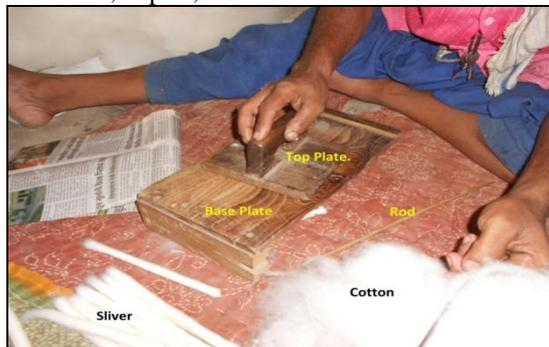
Fig 3. - Recent manual method of producing sliver (Pelu).
