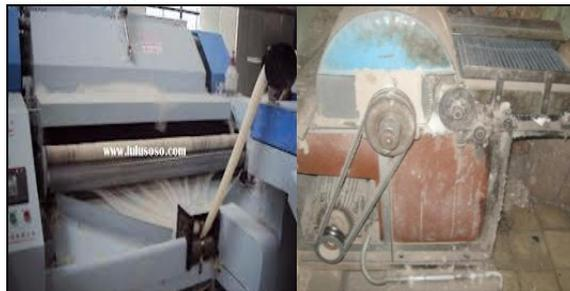
Fig 2. - Carding Machine use in Textile Industry and Pinjanalaya Carding Machine
