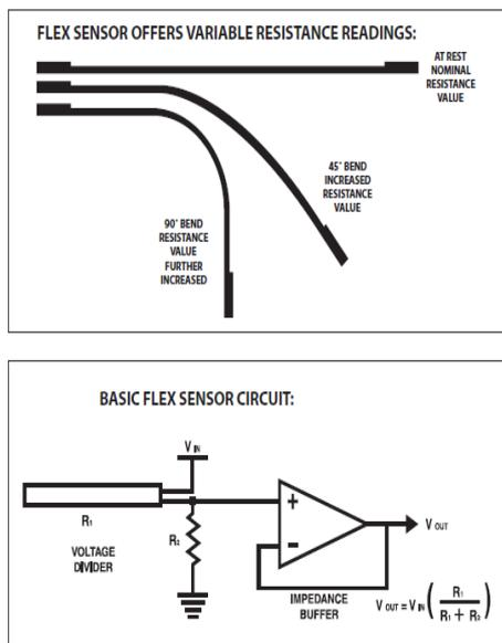
Fig.4: Circuit Diagram of Flux Sensor
