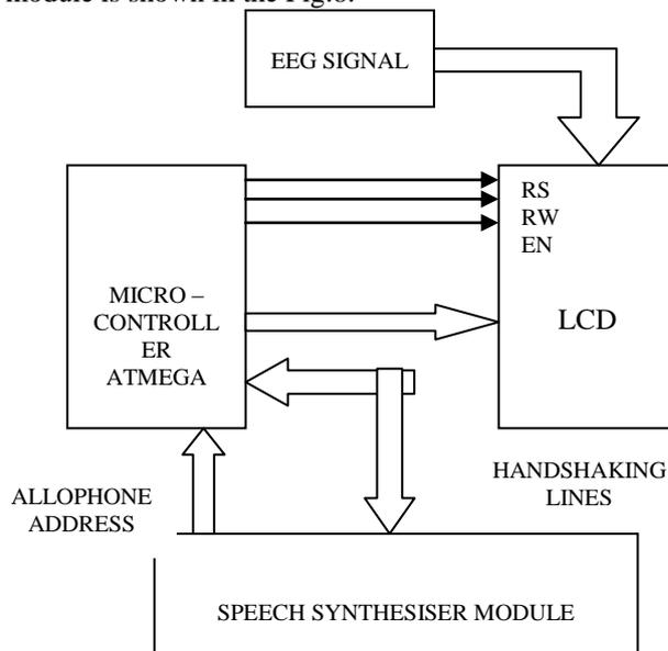
Fig. 8: Block Diagram LCD Display Module
