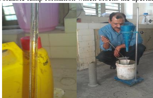
Fig. 1 Marsh Cone Test In Process
