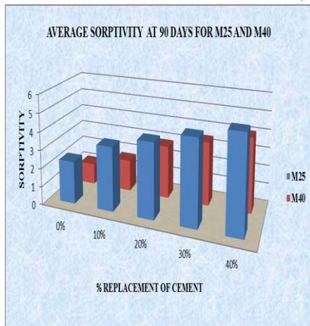
Fig. 5: % Replacement of Cement versus Sorptivity
