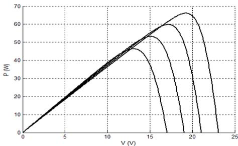
Fig (2) PV Characteristic of Solar Panel
