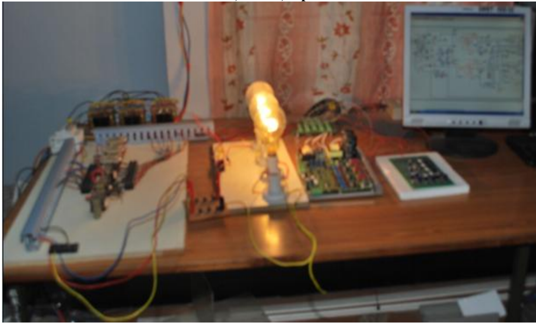
Fig.16 Hardware set-up of Shunt Active Power Filter
