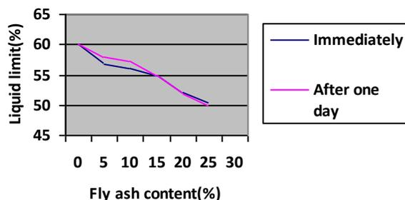
Figure 5 Variation of Liquid limit with Fly ash
