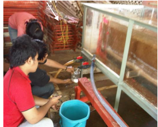
Fig. 3. Measures Water Out From Spill Way (Over Flow)
