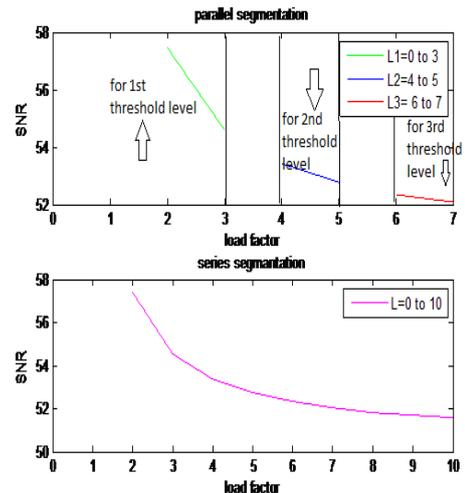
Fig.5 SNR as Function of Load Factor Where Thresholds are Even Segmented and Series Segmented at 64 Kbps
