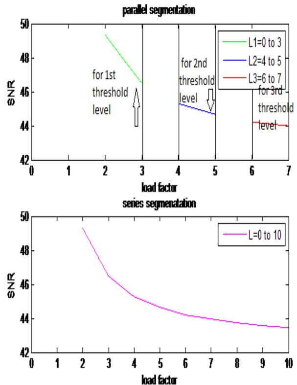
Fig.6 SNR as Function of Load Factor Where Thresholds are Even Segmented and Series Segmented at 144 Kbps
