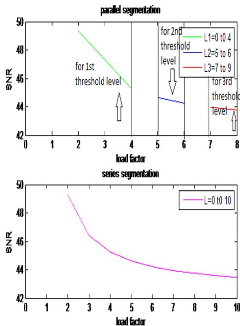
Fig.8 SNR as Function of Load Factor Where Thresholds are Odd Segmented and Series Segmented at 144 Kbps
