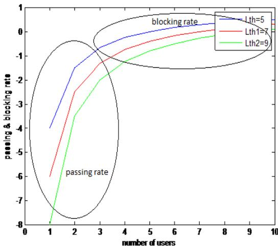
Fig.4 - Call Passing and Blocking Rate Where Threshold Load is Odd Segmented
