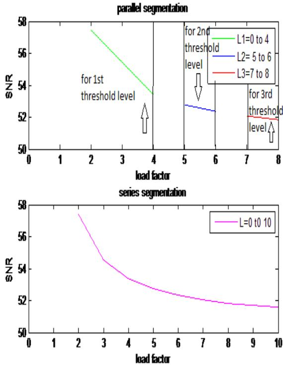
Fig.7 SNR as Function of Load Factor Where Thresholds are Odd Segmented and Series Segmented at 64 Kbps
