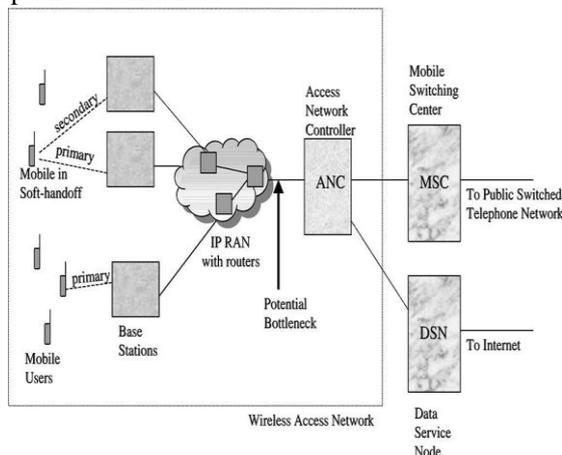
Fig.1. Wireless Access Network with IP RAN
