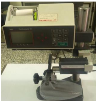
Fig 4. The Tool Used For Surface Roughness Measurement
