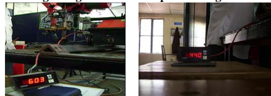
Fig. 7 & Fig. 8 Maximum Temperature_Trial1_at 5mm and Trial 2 at 15mm Distance From Centre of the Plates Respectively
