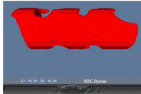
Fig.11 Iteration 4: Sloshing Of LPG in A Tank with Two Modified Baffle Showing Peak Amplitude of Fluid
