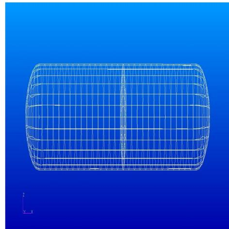
Fig.5 Meshing of LPG Tank with Full Enclosed Baffle at the Centre
