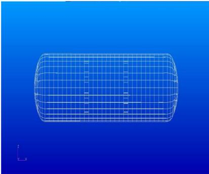
Fig. 6 Meshing of LPG Tank with Two Modified Baffles
