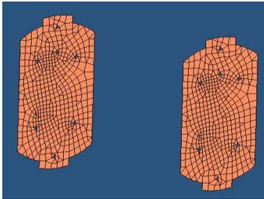
Fig. 7 Meshing of Modified Baffles
