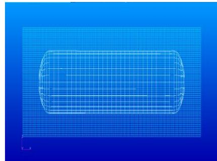
Fig.4 Meshing of LPG in Unbaffled Tank
