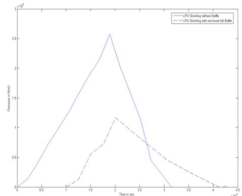
Fig.12 Comparison of LPG Sloshing Without Baffle and With Enclosed Full Baffle
