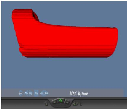
Fig. 8 Iteration 1 Sloshing of LPG without Baffle in Front View
