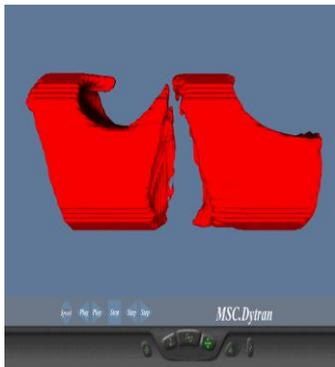
Fig.9 Iteration 2: Sloshing of LPG in a Tank with Enclosed Full Baffle at Initial Stage
