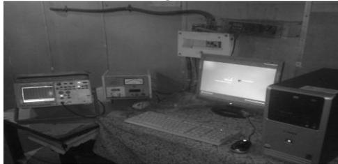
Fig. 4 Set Up For Partial Discharge Measurement
