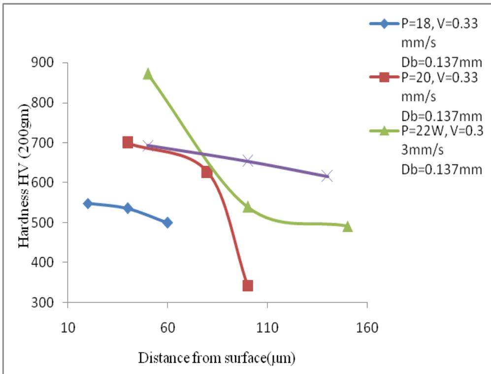
Fig. 6: Hardness Profiles in Samples Processed Under Different Processing Speeds
