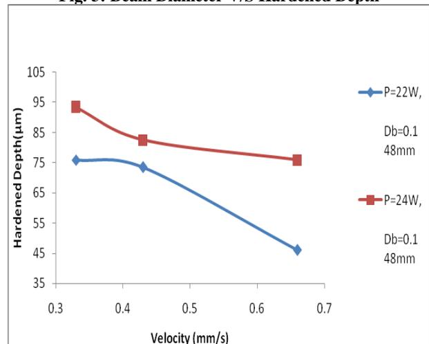
Fig. 4: Velocity v/s Hardened Depth
