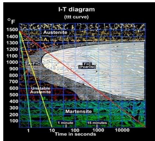
**Fig. 2: TTT Curve – Principle for Martensite Formation**
