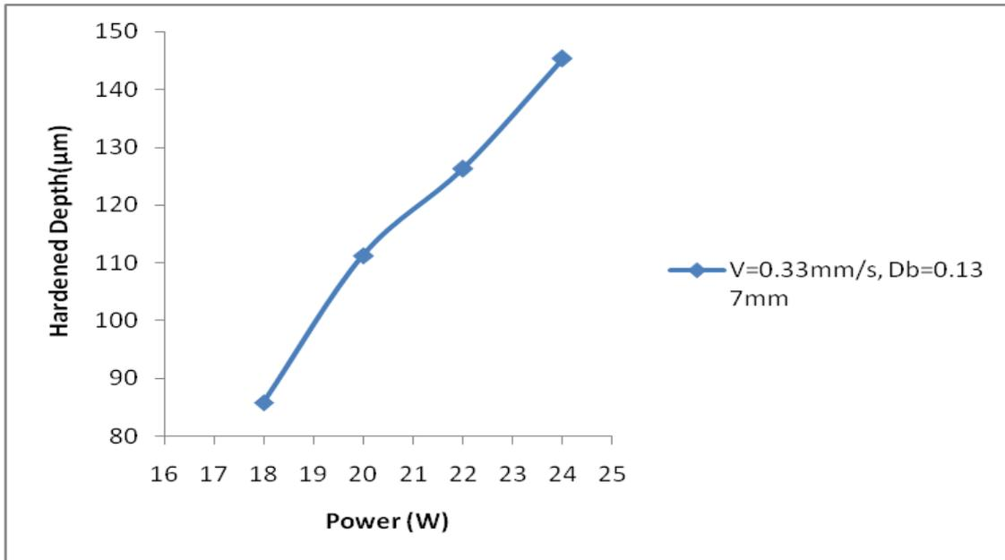
Fig. 5: Power v/s Hardened Depth
