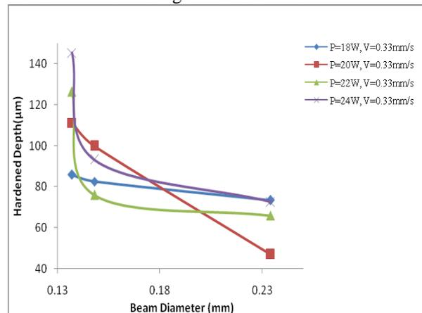
Fig. 3: Beam Diameter V/S Hardened Depth
