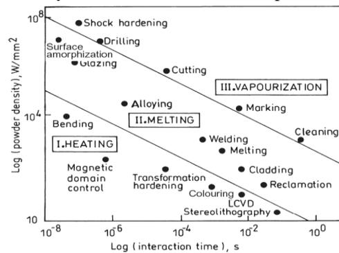
**Fig. 1: Different Laser Material Process in Terms of Power Density as Function of Interaction Time**
