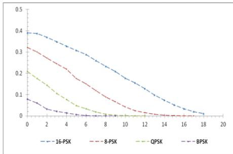
**Fig 2: Plot of SNR value in dB to BER(X axis SNR & Y axis BER).**
