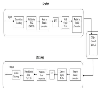
**Fig 1: Block Diagram OFDM (Sender and Receiver)**
