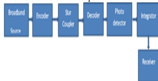
**Fig 1: Block Diagram of Optical CDMA system**
