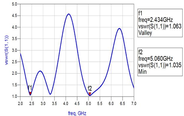
**Fig. 5 The Simulated VSWR of The Proposed Dual Band Monopole Antenna Designed In ADS**
