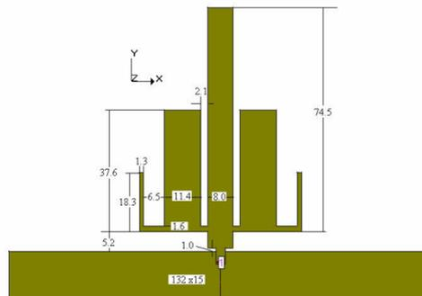
Fig. 1 Geometry of the Proposed Dual Band Monopole Antenna
