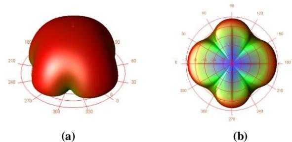
**Fig. 10 3-D Radiation Pattern of the Dual-band antenna at 5.1 GHz (a) Bottom View and, (b)**
