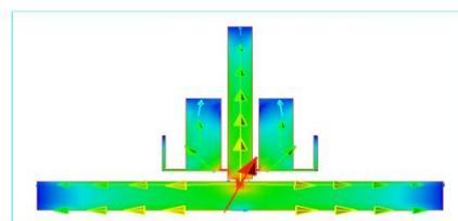
Fig. 3 Current Distribution of the Proposed Dual Band Monopole Antenna Designed In ADS
