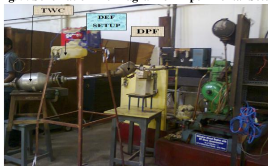
Fig. 10. DPF+TWC Converter +DEF Experimental Setup with Engine
