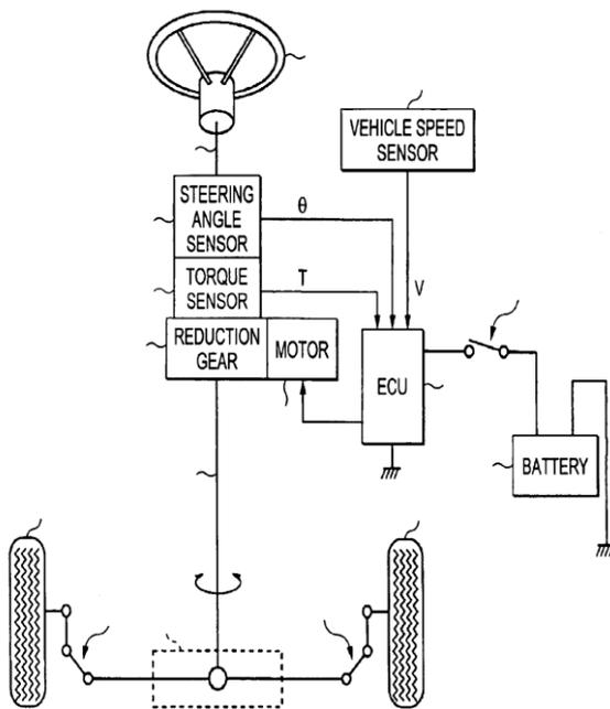
**Fig 1: Electrical Power Steering System**
