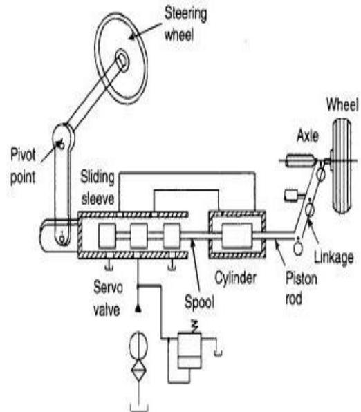
**Fig 2: Hydraulic Power Steering assembly**
