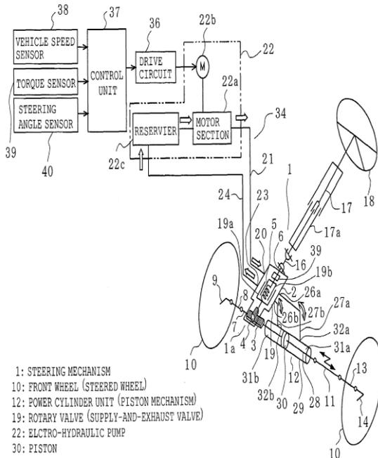
**Fig 3: Shows the Electro-Hydraulic Power Steering Model**
