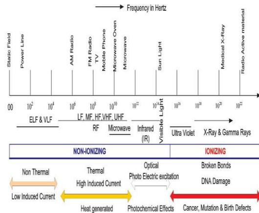
Fig 1. Electromagnetic Spectrum
