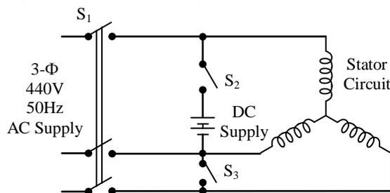
Fig. 3. D.C. Injection Braking
