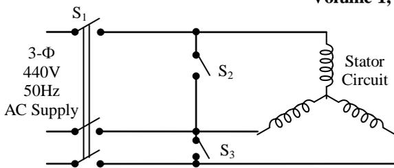
Fig. 4. Magnetic Braking
