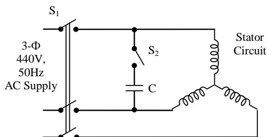
Fig.2. Capacitor Braking
