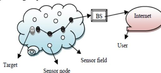
Fig 1 Sensor Nodes in a Sensor Network
