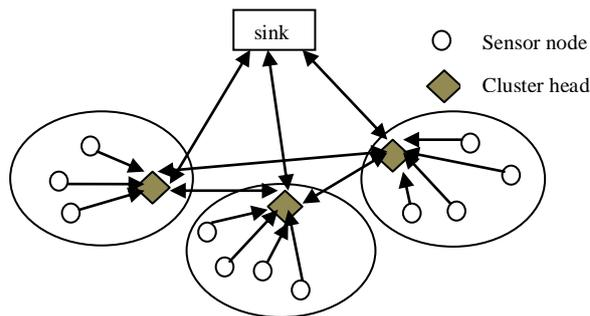
Fig 8 Cluster based architecture
