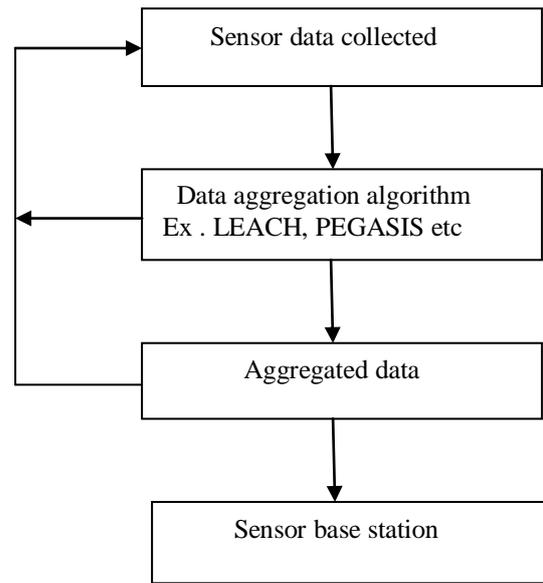
Fig 4 Data aggregation flowchart
