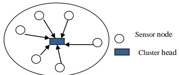
Fig 5 Centralized architecture
