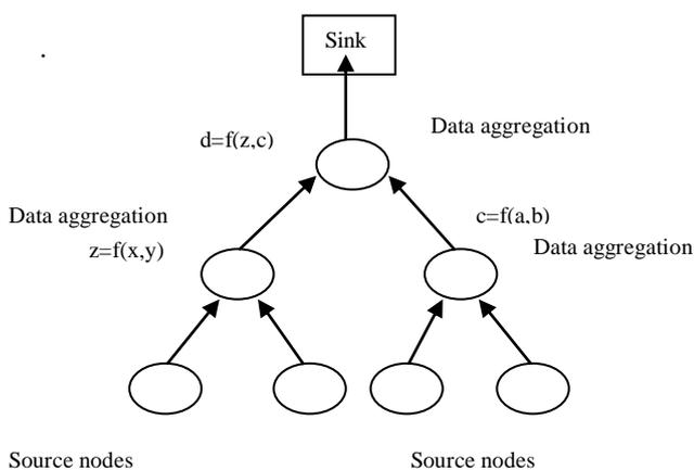
Fig 7 Tree based architecture
