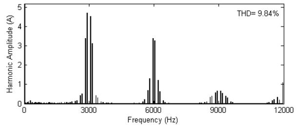
**Fig.6 Harmonic Spectrum of line current for 2-level SVPWM based DTC along with THD**
