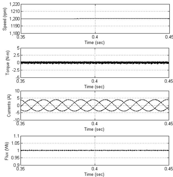
**Fig. 12 Simulation results of 5-level SVPWM based DTC: steady-state plots of speed, torque, currents and flux at 1200 rpm**
