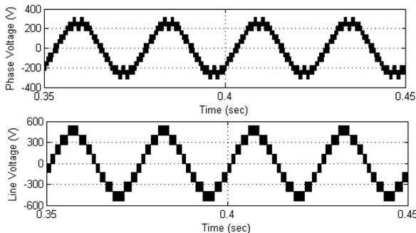
**Fig. 13 Simulation results of 5-level SVPWM based DTC: steady state plots of phase and line voltages**
