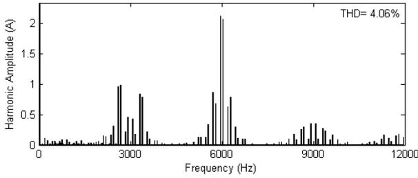
**Fig.10 Harmonic Spectrum of line current for 3-level SVPWM based DTC along with THD.**
