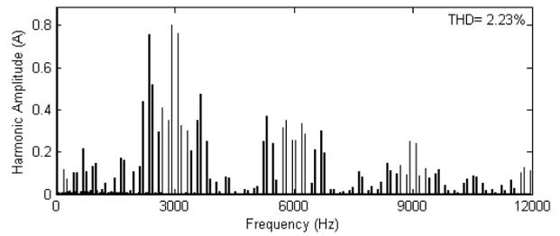
**Fig. 14 Harmonic Spectrum of line current for 5-level SVPWM based DTC along with THD**
