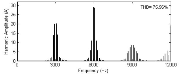
**Fig.7 Harmonic Spectrum of line voltage for 2-level SVPWM based DTC along with THD**
