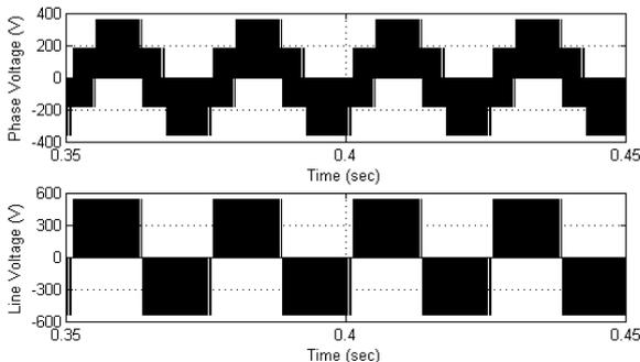
**Fig.5 Simulation results of 2-level SVPWM based DTC: steady state plots of phase and line voltages**
