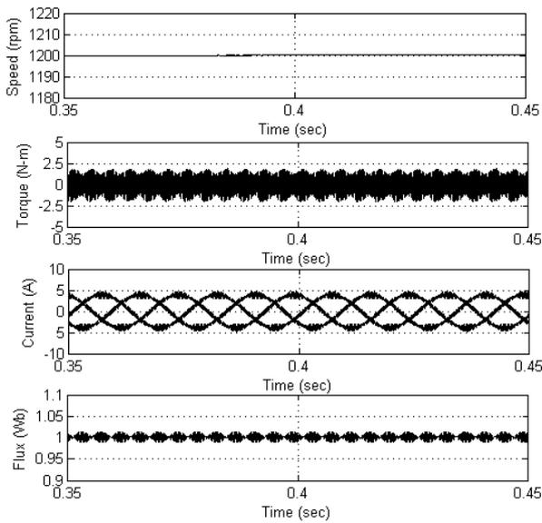
**Fig.4 Simulation results of 2-level SVPWM based DTC: steady-state plots of speed, torque, currents and flux at 1200 rpm**
