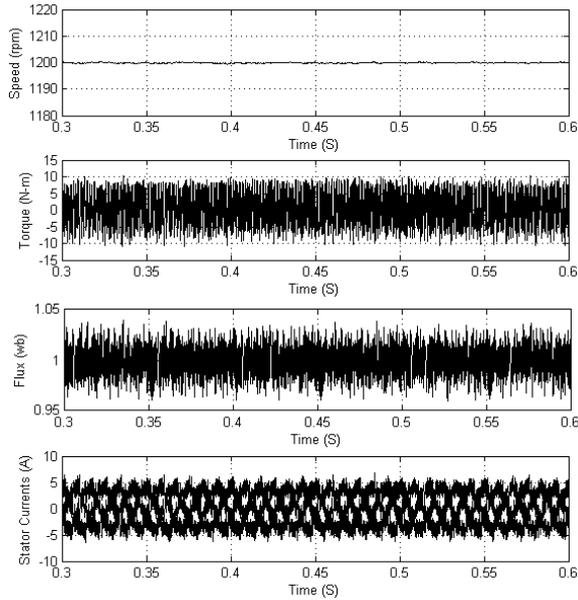
**Fig.3. Simulation results of Conventional DTC: steady-state plots of speed, torque, currents and flux at 1200 rpm**
