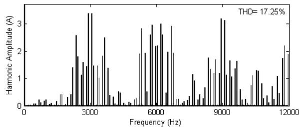
**Fig. 15 Harmonic Spectrum of line voltage for 5-level SVPWM based DTC along with THD**
