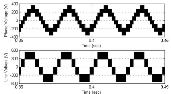
**Fig.9 Simulation results of 3-level SVPWM based DTC: steady state plots of phase and line voltages**
