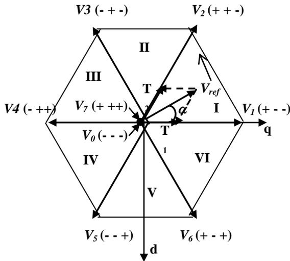
Fig. 1 Voltage space vectors produced by an inverter
