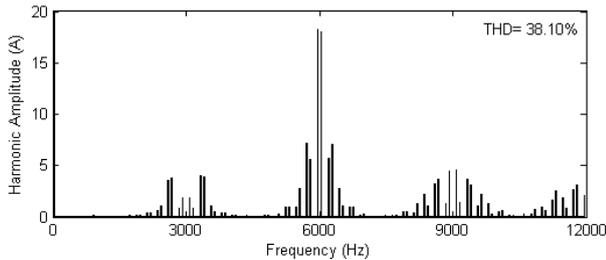
**Fig. 11 Harmonic Spectrum of line voltage for 3-level SVPWM based DTC along with THD.**
