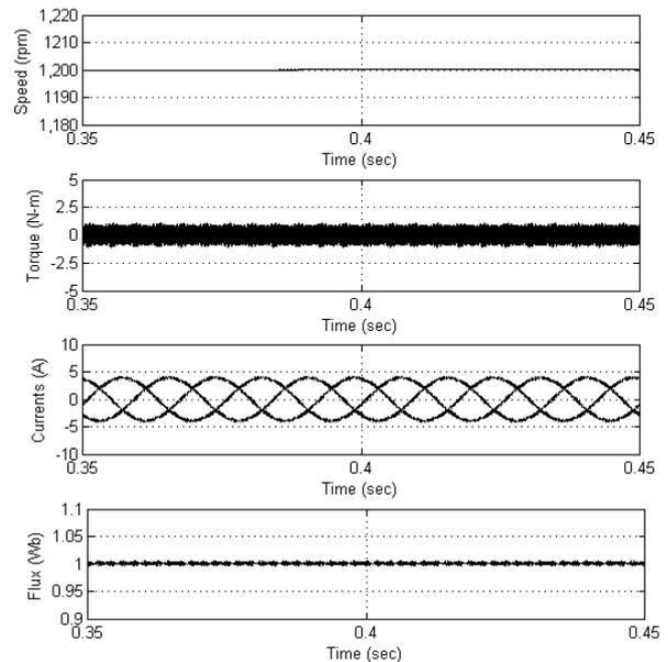
**Fig.8 Simulation results of 3-level SVPWM based DTC: steady-state plots of speed, torque, currents and flux at 1200 rpm**
