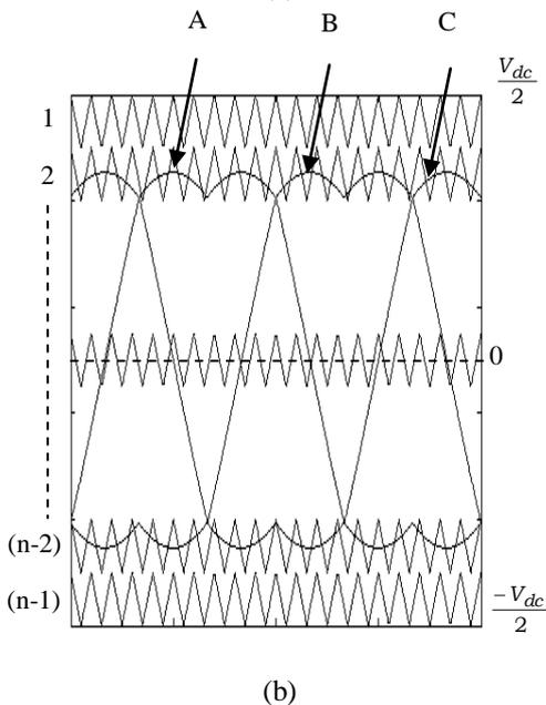
Fig.2 triangular carrier and reference signals (a) n-level PWM scheme where n is even (b) n-level PWM scheme where n is odd
