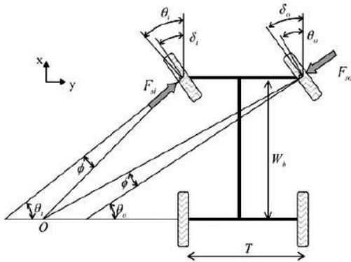
Fig. 2: Center of turning circle [3]
