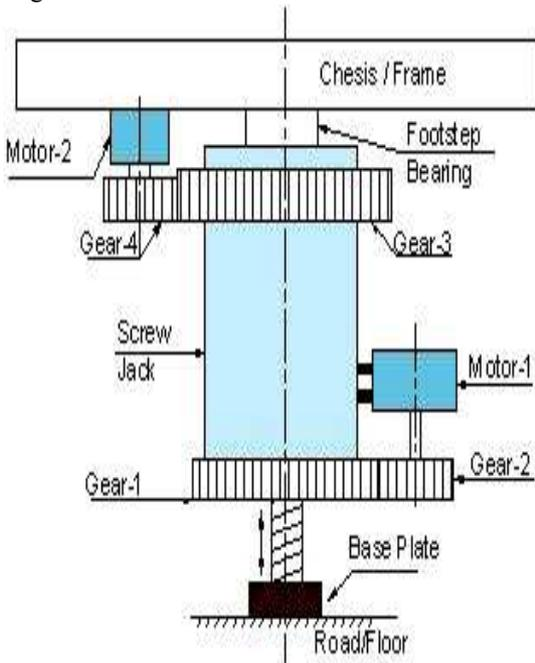
Fig. 6: Lifting and turning system
