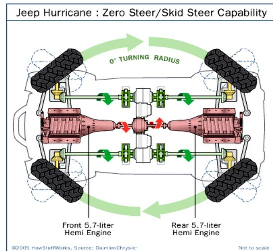
Fig. 5 Zero turning radius mechanism in zeeep hurican [5]
