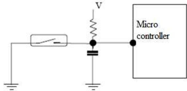
Fig. 3: Interfacing of Reed Switch to controller
