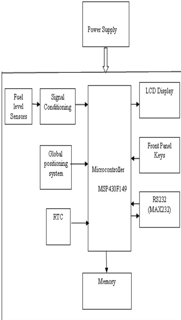
Fig. 2: Block Diagram
