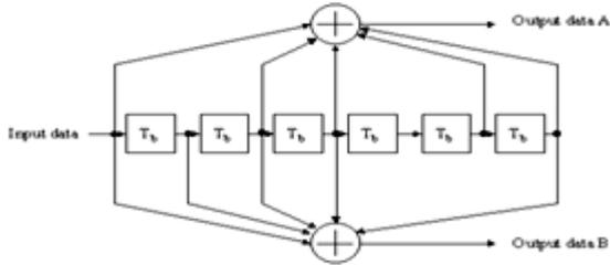
Fig.5 convolutional encoder [5]
