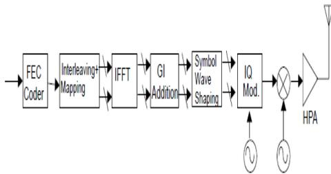
Fig. 3 WLAN (802.11a) transmitter [5]
