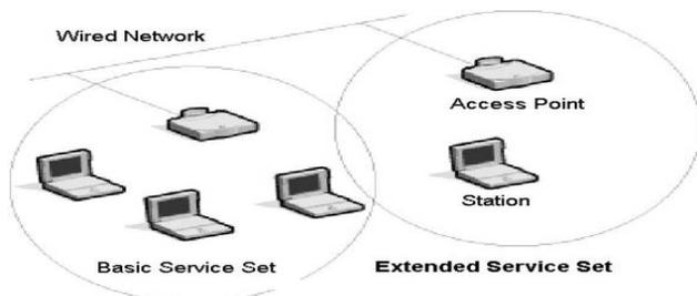
Fig. 1 .WLAN Architecture
