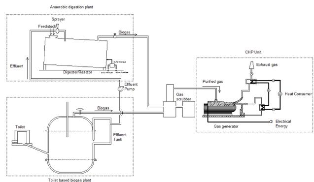
Fig.3. Design of proposed integrated market waste management plant
