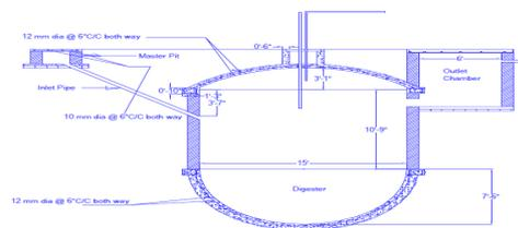
**Fig 1: Design of a Biogas plant considering 300 users per day (designed by author)**
