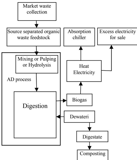
Fig.2. Flow Diagram of Proposed Digestion Process (Regenerated From [8])
