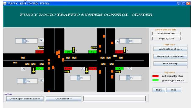
Fig. 3 .The simulated fuzzy logic traffic control system [13], [14]
