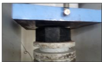
Fig.5 Compression test on pavers
