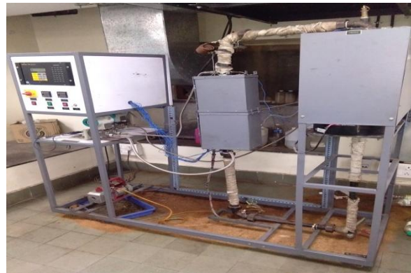
Fig. 2. Set up of closed loop thermosyphon
