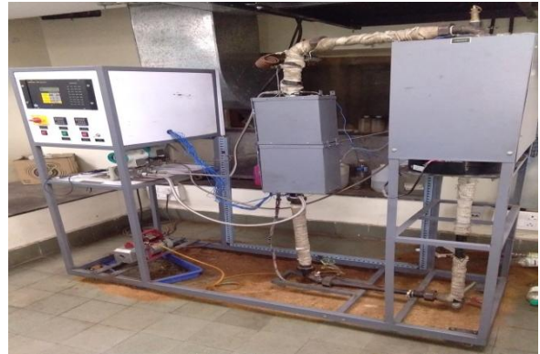
Fig. 2. Set up of closed loop thermosyphon
