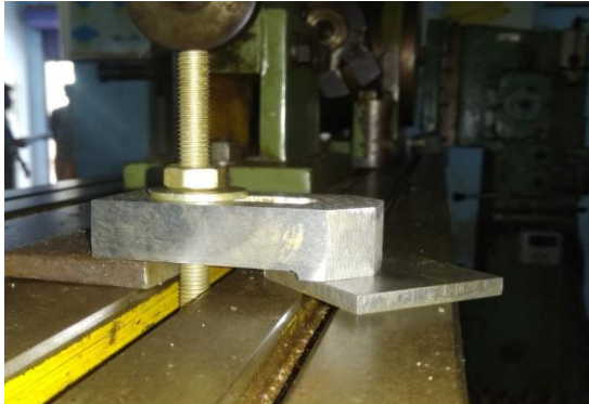
Fig: 22 Work piece clamped on machine table without fixture
