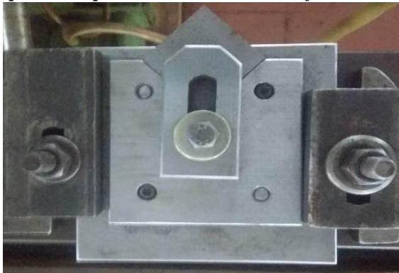
Fig: 23 Work piece clamped on machine table with fixture
