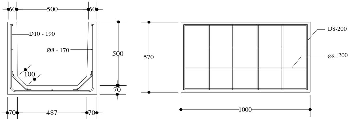
Fig 7. Detail of reinforcement
