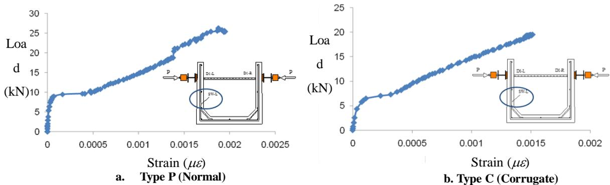
Fig 15. Load-strain at steel bars
