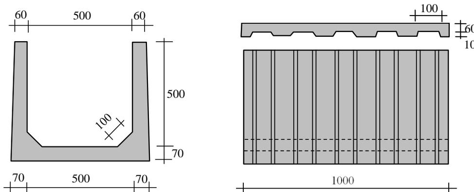
Fig 6. Dimension of Type C (Corrugate)
