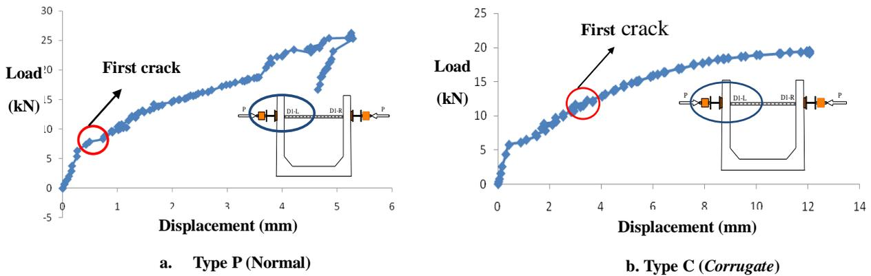
Fig 13. Load-displacement relationship
