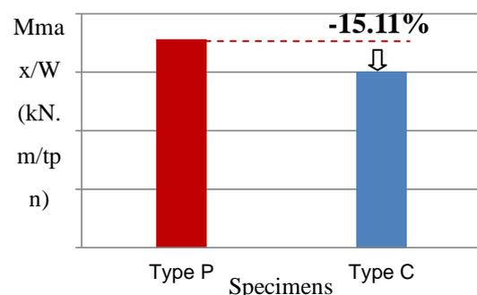
Fig 12. Ratio of moment capacity to weight
