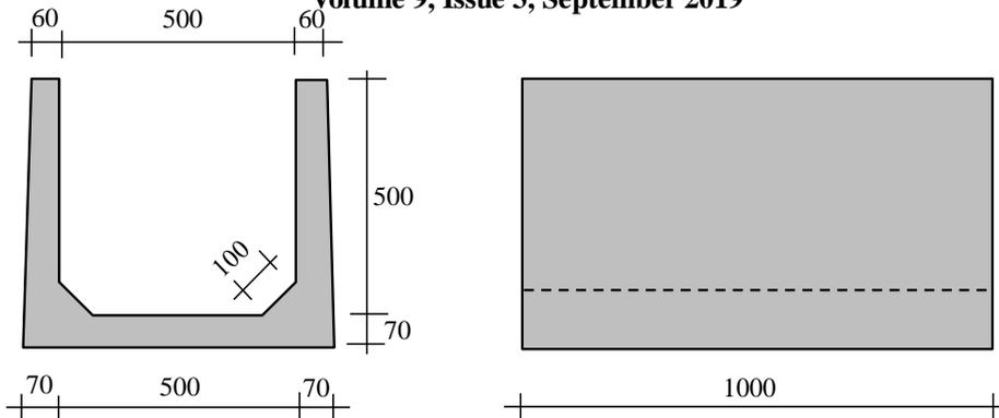
Fig 5. Dimension of Type P (Normal)
