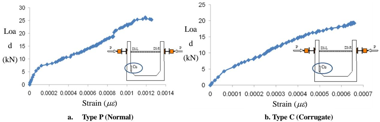
Fig 14. Load-strain at concrete
