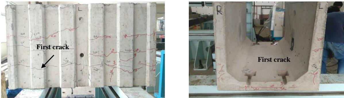
Fig 16. Crack pattern
