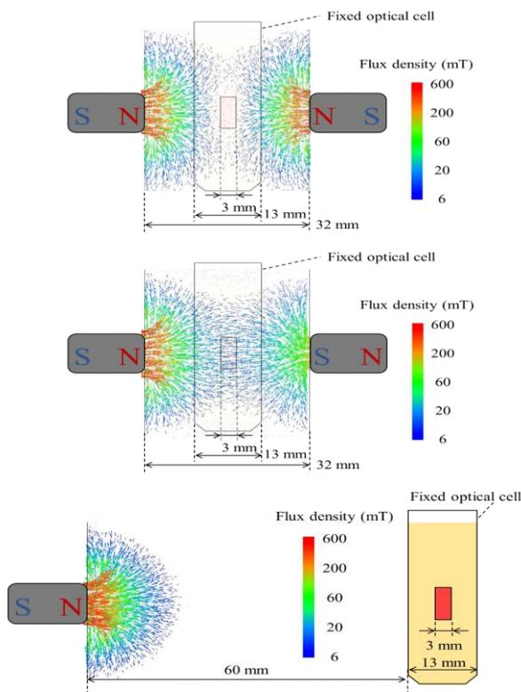
Fig. 4: Simulation of magnetic field lines: (a) repelling direction of the magnet, (b) attracting direction, and (c) one magnet
