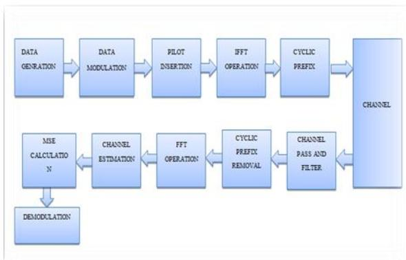
**Fig.2 Block Diagram of a Base-band OFDM**
