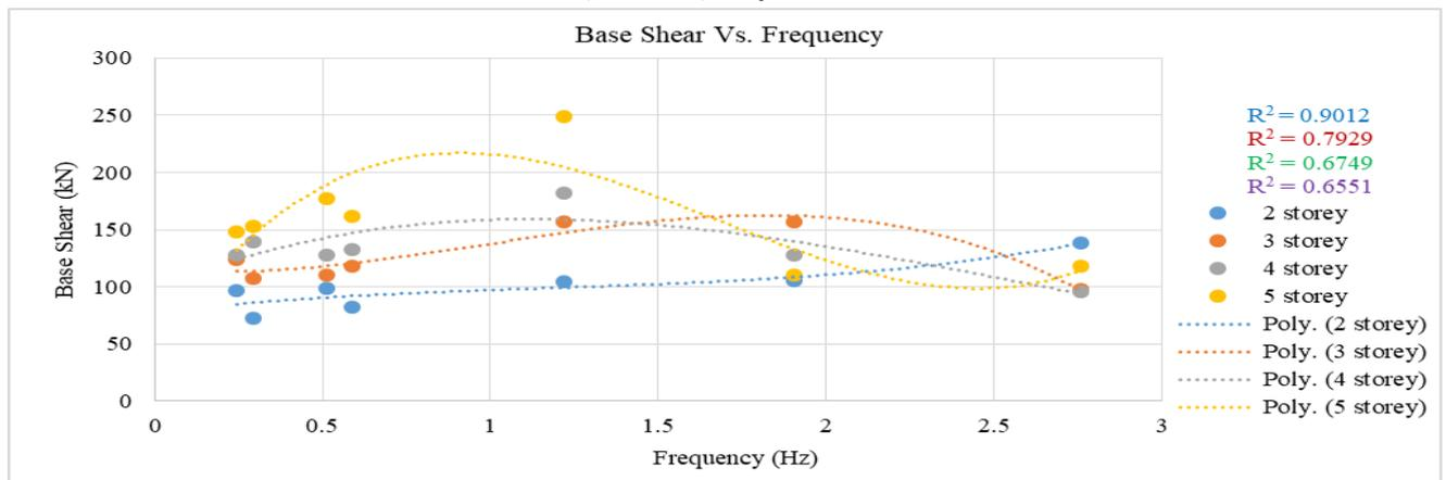
Fig. 6. Base shear of buildings with varying predominant frequency of ground motion
