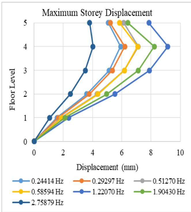
Fig. 3. Maximum storey displacement of four storey building with staircase cover due to ground motion of different predominant frequency
