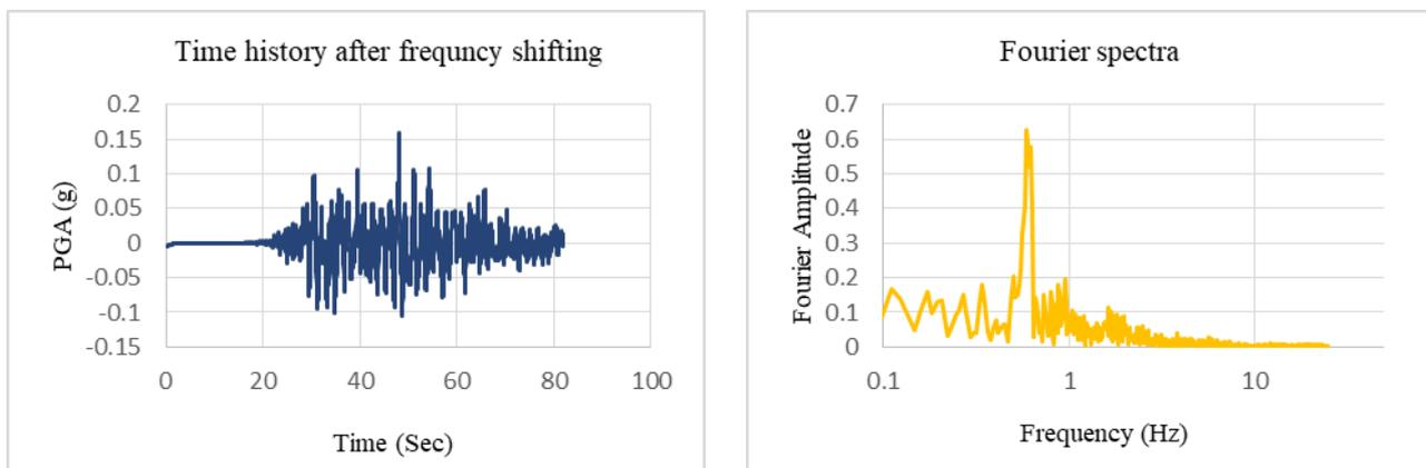
Fig. 2. Time history and Fourier spectra of Gorkha earthquake after frequency shifting, predominant frequency 0.58594 Hz
