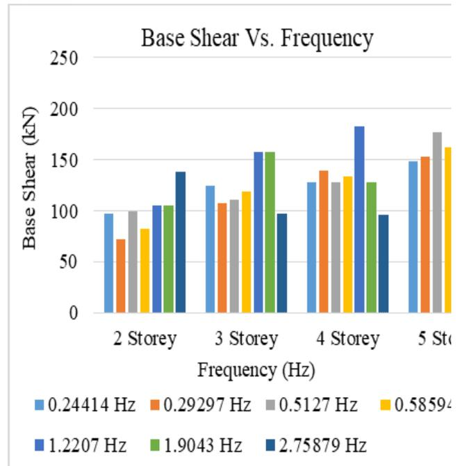
Fig.5. Base shear of buildings with varying predominant frequency of ground motion
