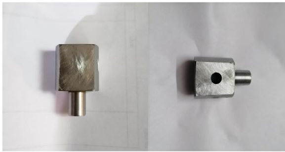
Fig 31: Before and after Drilling Operation
